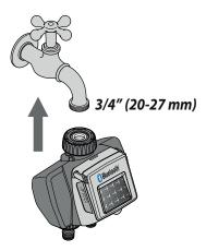
Fit the timer to a cold water tap. The spout of the tap should have a 3/4" male thread (if not, use an adaptor).
