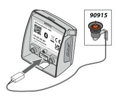
Insert the Rain Sensor connector. The sensor will be active immediately. Warning: if neither the jumper nor the Rain Sensor connector are connected, the timer will only run manual irrigation programmes and not any automatic irrigation programmes.
