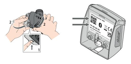
Enter the numerical code (PIN) or scan the QR code. This information is on the back of the control unit: disconnect it from the timer to access it.
