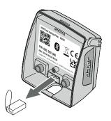
Remove the bridge connector on the timer.
