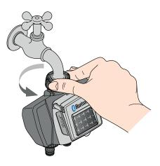
Screw the clamp collar of the 3/4" female fitting onto the tap.
