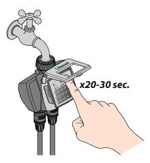
If the timer behaves anomalously, it can be reset. The reset will NOT cancel the programmes set, nor the date and time, but will only restart the circuit board.
