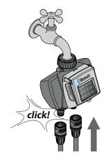
Connect the irrigation lines to the timer connector using Quick-Click System fittings or 3/4" threaded fittings.
