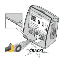
With the help of small pliers, break the plastic plug for preparing the slot of the Rain Sensor cable.
